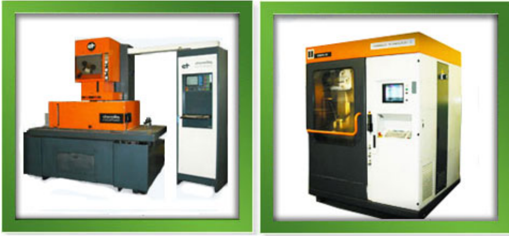
Charmilles Robofill 310 – Programmable 5-Axis control; X=15.75", Y=9.85", Z=15.75" travel, up to 30deg. Taper, .0001 Tolerance.
